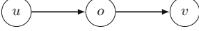
Fig. 1. A simple topology with 3 operators. The size of state of o is set to one tenth of the data rate, \psi(o) = \frac{1}{10}r(o) .
